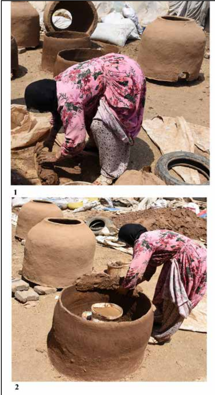
Figure 8: Making a tandoor using long slab (short band) construction with elements of coil rolling movements (Diyarbakir area, Türkiye).
