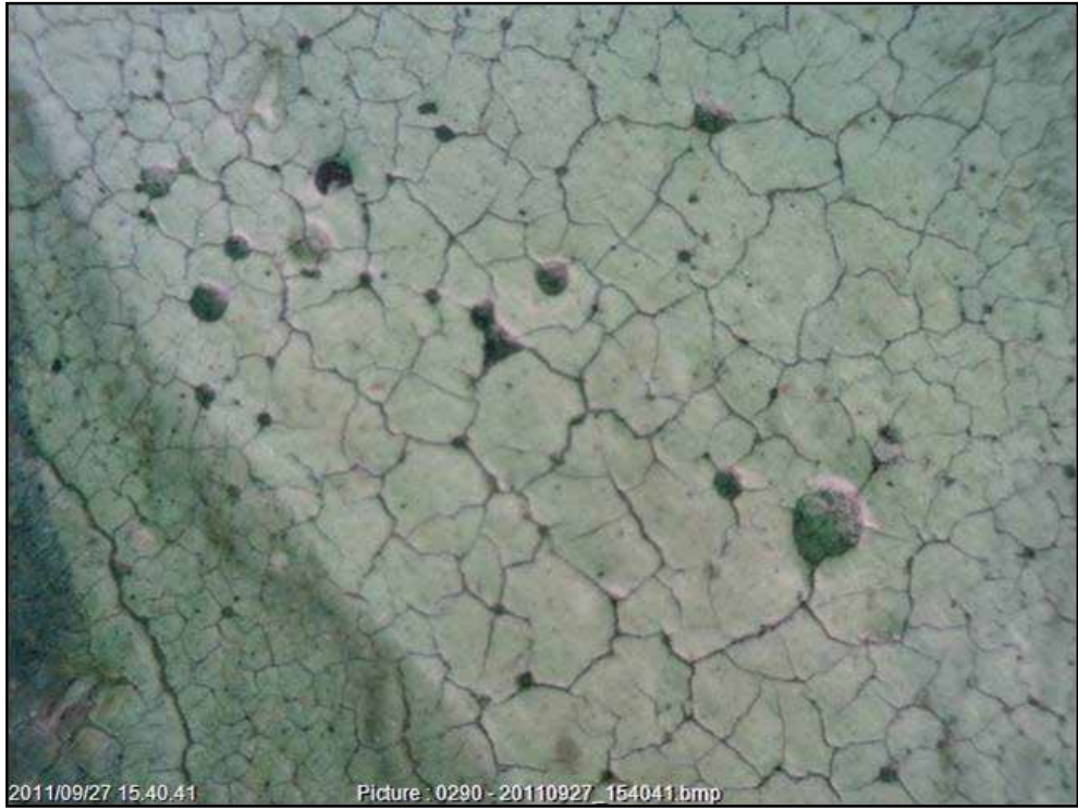
Figure 3. New Tokalı Church, south side. Detail of micro-cracking (craquelure) in the paint layer (50x magnification).
