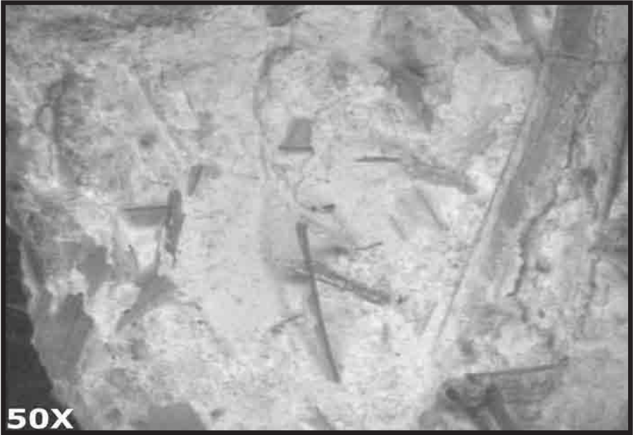
Fig. 5: Şahinefendi, Forty Martyrs Church, south nave, unit \beta II2. White plaster with straw, magnification 50x
