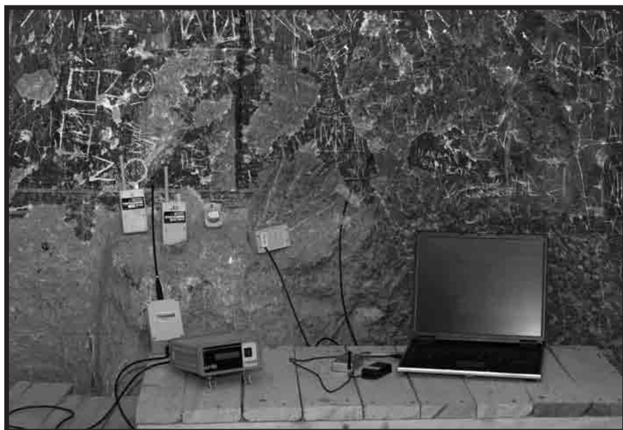
Fig. 8: Şahinefendi, church of the Forty Martyrs, pilot system for monitoring at a distance the micro-climatic conditions
