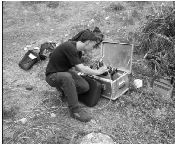
Fig. 6: 2-D resistivity imaging along one of the 5 profiles
