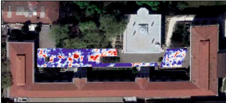
Fig. 2. GPR results from the courtyard of the Istanbul Archaeological Museums. The anomalies may relate to complex systems of cisterns and water channels (C. İmren and B. Karadöller). Fig. 3. Courtyard of the archaeological museum in Istanbul, with the updated location of cisterns and channels (C. İmren, B. Karadöller, Ç. Özkan Aygün)
